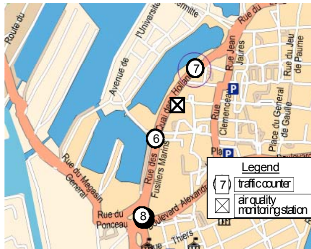
Figure 2: Spatial configuration of monitoring equipment
