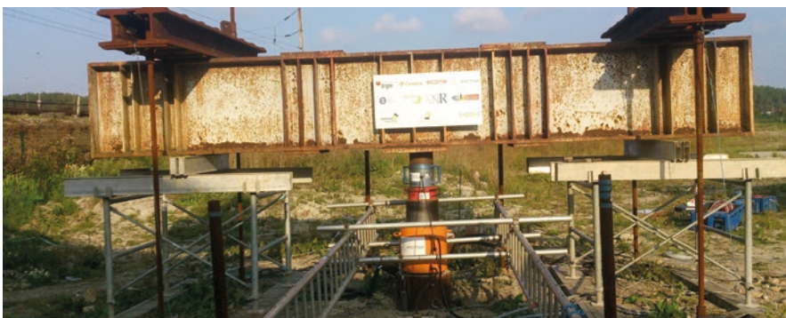
Loading test for a geothermal pile
