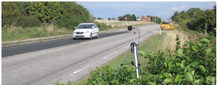
Measurement of rolling noise (ISO 11819-1 method) when passing on the poro-elastic test board of Kalvehave in Denmark
