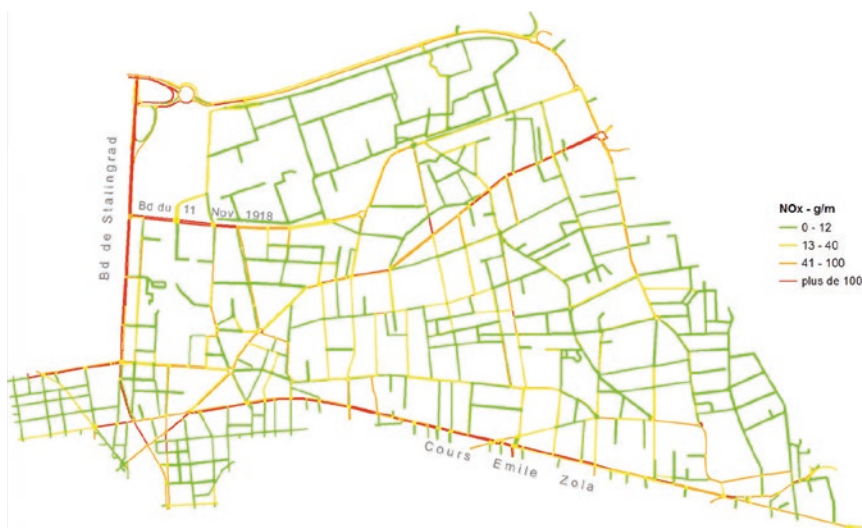
Emissions of nitrogen oxides as estimated with the Copert model over a period of 15 min at rush hours
