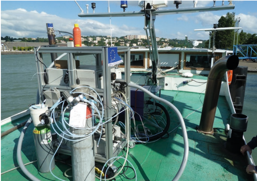
Instrumentation on the rear deck of a CFT (major river transport operator) ship to measure pollutant emissions
