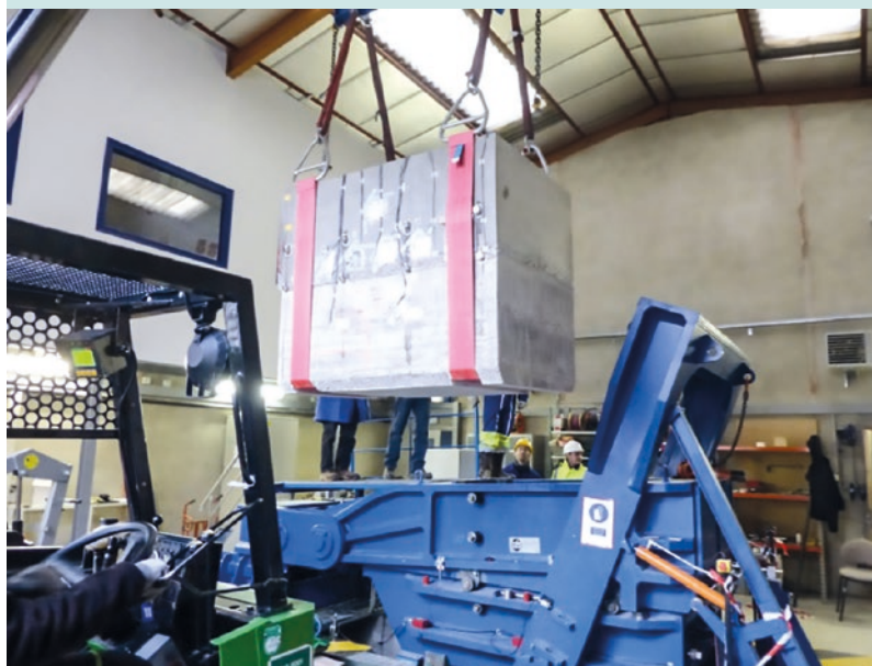
5-tonne granite-concrete test cube placed in the large-scale Casagrande shear test apparatus at the Cerema centre in Bron, prior to testing
