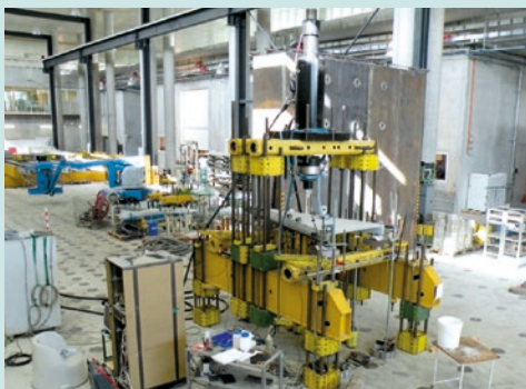
Closed frame mount for the bending stress test on the UHPFRC concrete triangular plates
