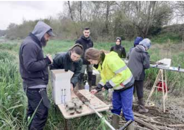
Cutting up a sediment core taken from the Loire. © Johnny Gasperi
